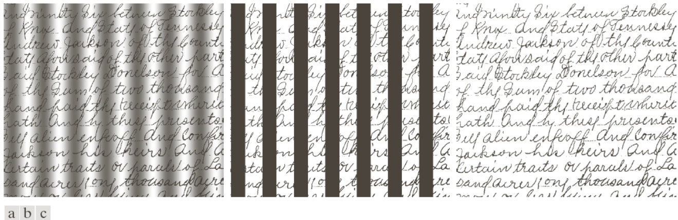
FIGURE 10.50 (a) Text image corrupted by sinusoidal shading. (b) Result of global thresholding using Otsu's method. (c) Result of local thresholding using moving averages.
