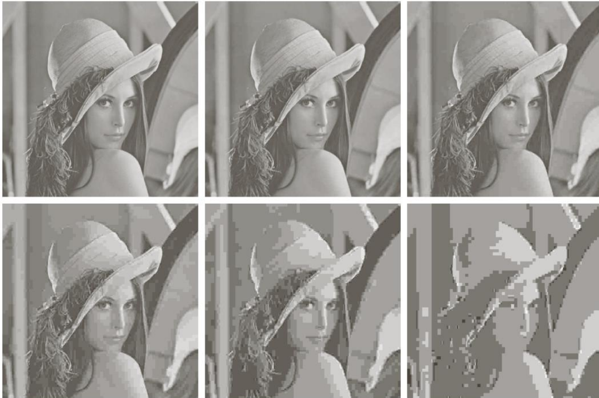
FIGURE 8.31 Approximations of Fig. 8.9(a) using the DCT and normalization array of Fig. 8.30(b): (a) Z , (b) 2Z , (c) 4Z , (d) 8Z , (e) 16Z , and (f) 32Z .
